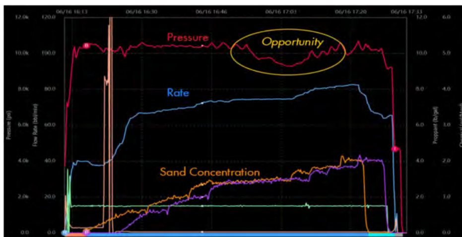
Figure 2—A typical frac treatment stage showing an opportunity where rate and/or sand concentration may have been increased earlier in the stage by responding quickly as pressure stabilized and fell below upper limit.
